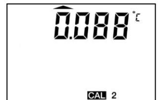
The arrow on the top indicates that the instrument is working in the Filter-Mode.
