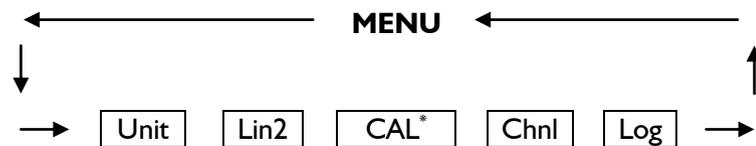
\*The calibration is hidden when the instrument has been calibrated at Isotech, see page 6 for details.
