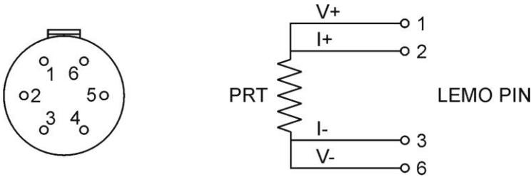
Three wire probes can be connected, link pins 1 and 2.
