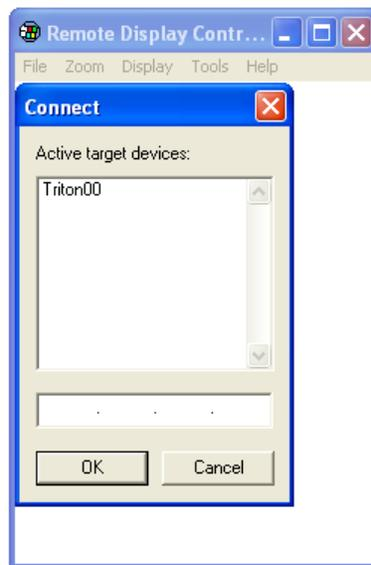
Click on the required device (“Triton00” in the above example) and then click OK, cerhost will then establish a connection and display the screen as it appears on your milliK:
