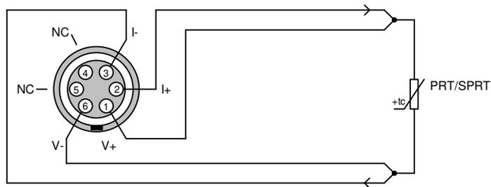
If the PRT is supplied with a 3-wire connection, the current and common wires should be of the same resistance (of same length and gauge) and connected directly to I+ and I- (pins 2 and 3) and a link that carries no current should be made from pin 1 to pin 2 (see section 3.1.3):
