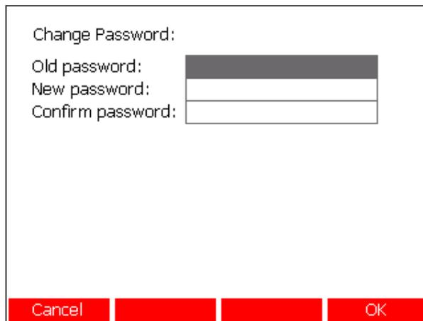
Use the **↑****↓** keys to select each password entry in turn and then press the **↵** key to open a soft keyboard and enter the value. The ‘New Password’ and ‘Confirm Password’ entries must be identical (and at least 4 characters long) in order to proceed.
