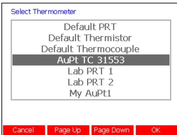
Select the thermometer and set the remaining parameters in the **Settings** Window. A typical configuration for a calibrated SPRT would be:
