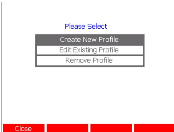
Use the **↑↓** keys to select whether you wish to create, edit or delete a profile and then press the **↵** key to open the ‘Temperature Profile’ Window:
