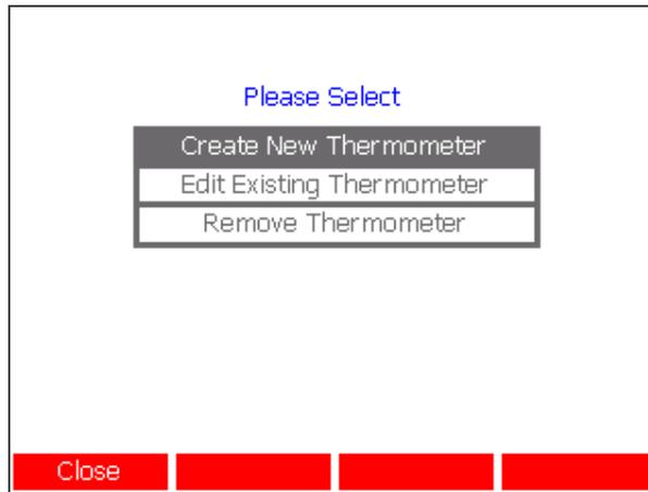
Use the **↑↓** keys to select **Create New Thermometer** and press the **↵** key to open the 'Thermometer' Window:
