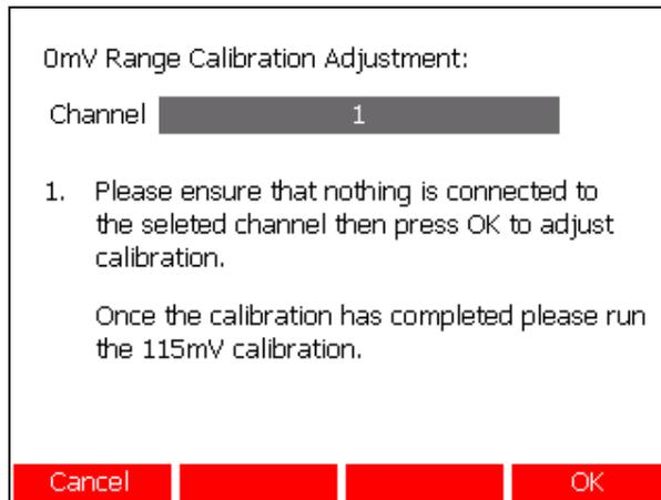
Press the **OK** (F4) key to start the calibration adjustment. Once started, the calibration adjustment process cannot be aborted. Repeat the procedure on Channel 2.
