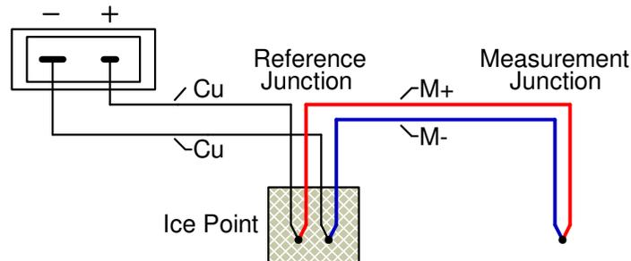
When using a thermocouple with the reference junction in an ice point, the 'Reference' parameter in the **Settings** Window should be set to 0°C (see section 3.3.4). Also, you MUST use a copper miniature thermocouple connector in order to avoid introducing unwanted additional thermal EMFs.
