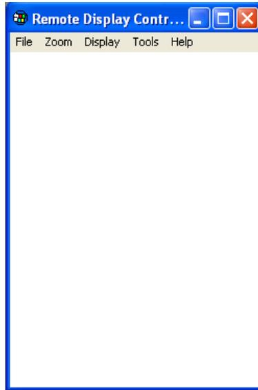
Click on “File” and then “Connect...” to establish connection with the milliK, a ‘Connect’ Window will then appear and after a few seconds it will show a list of available devices that includes the milliK (the milliK will be listed as “Tritonxx” where xx is a number assigned to the milliK in case you have more that one connected to the LAN):
