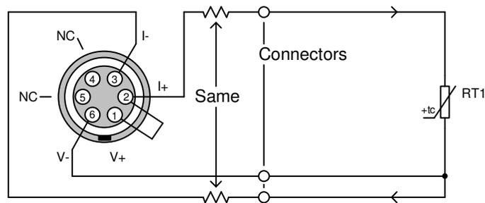
This can be achieved by using the same gauge and length of wire for the I+ and I- leads. Use the lowest resistance wire (that is mechanically suitable) so as to minimise the resistance of the extension connections and therefore minimise any error from the imbalance in their resistance.
