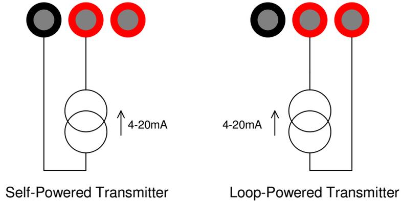
The 4-20mA system and 24V supply are isolated from both the measurement system of Channels 1 and 2 and from the digital interfaces in order to optimise immunity to external (common-mode) noise sources.
