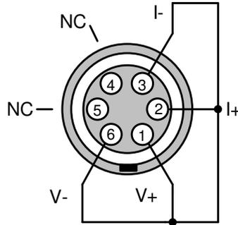
It is important that none of the current flowing between I+ and I- flows along the short circuit between V+ and V-. There should only be a single link between the voltage and current circuits, as shown.
