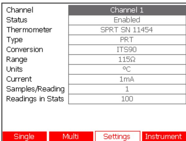
Once you have configured the milliK to work with your PRT/SPRT, press either the **Single** (F1) or **Multi** (F2) keys to view the measurements:
