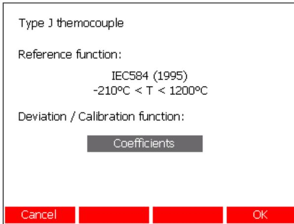
Use the **←** **→** keys to toggle ‘Deviation / Calibration function’ between “Coefficients” and “Data Pairs”. Press the **⏏** key to open a soft keypad and enter the required data.
