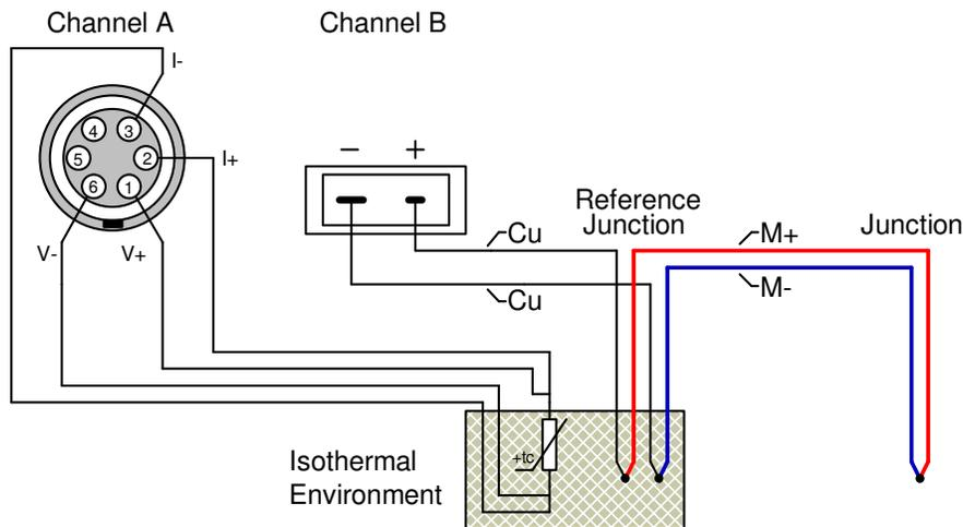
When using a thermocouple with external reference junction compensation, the ‘Reference’ parameter in the **Settings** Window should be set to the channel used to measure the reference junction (see section 3.3.4). Also, you **MUST** use a copper miniature thermocouple connector in order to avoid introducing unwanted additional thermal EMFs. Only channels configured to measure temperature (i.e. having a Conversion defined) appear in the
