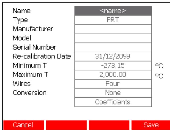
Use the **↑↓** keys to select each parameter in turn and press the **↵** key to open a Window and enter a value or select an option. A typical entry for an SPRT would be:
