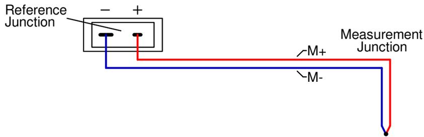
When using a thermocouple with internal reference junction compensation, the ‘Reference’ parameter in the **Settings** Window should be set to “Internal” (see section 3.3.4).
