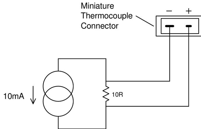
The connections from the 10Ω resistor to the thermocouple connector should be entirely in copper and should not involve intermediate connectors (to avoid thermal EMFs). Set the milliK to read this voltage by changing the parameters in the ‘Settings’ Window (see section 5.2.3 for details of settings).
