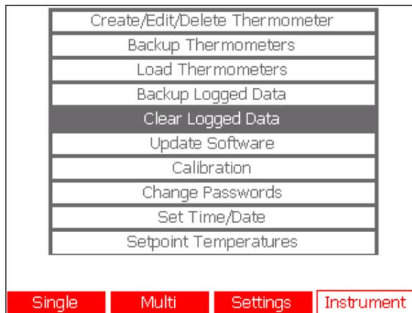
Press the **↓** key to clear the memory. The milliK will then display the number of files you are about to remove and will ask you to provide the password (see section 3.11) in order to proceed.
