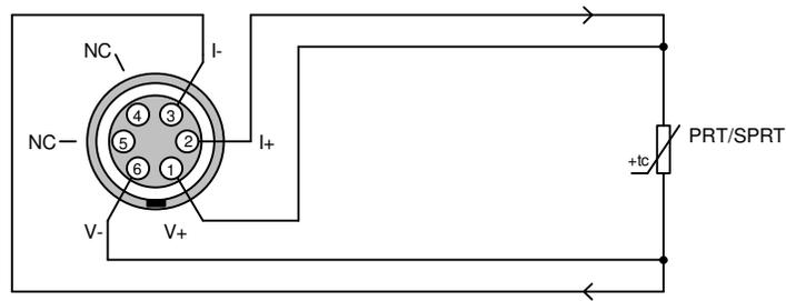
If the PRT is supplied with only a 2-wire connection, convert from 4-wire to 2-wire connection as close to the PRT as possible:
