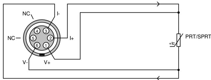
Since the current along the voltage sense wires is effectively zero, the milliK is able to measure the resistance of the PRT element without being affected by the resistance of the wires.
