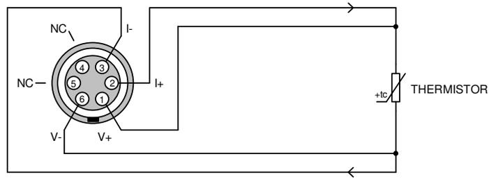
The relatively high resistance of thermistors means that they are used with much lower sense currents ( $2\mu\text{A}$  on milliK) than PRTs/SPRT and the effect of the cable resistance is much lower. Thermistors are therefore sometimes supplied with only 2-wire connections, in which case they can be connected to the milliK as follows:
