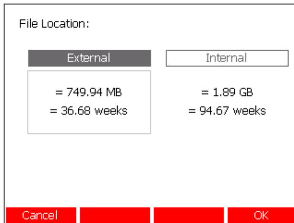
Use the **←** **→** keys to select whether to store the file to external or internal memory and then press the **OK** (F4) or **↵** keys to open a soft keyboard and enter a filename (a default filename generated from the date/time is suggested automatically):
