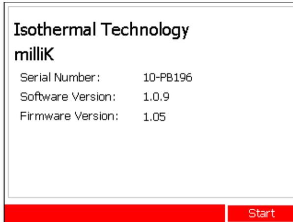
Press the right-hand function key below **Start** to proceed (or connect a USB keyboard or mouse and press F4 or click **Start**). The milliK software will then start and you will see the main Windows:
