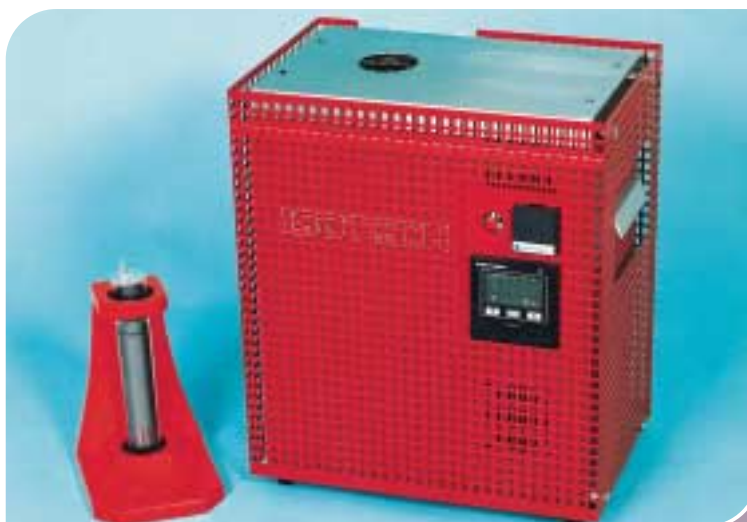
High Temperature Furnace for Aluminium, Silver, Gold or Copper Blackbody Fixed Point Cells
